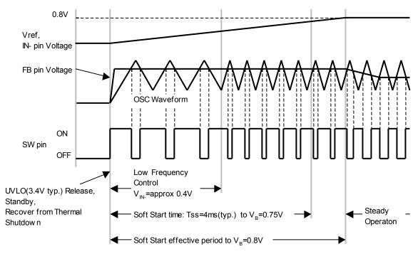
Fig. 2. Startup Timing Chart
