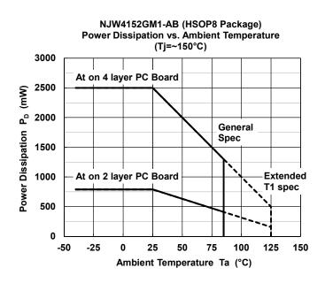
Mounted on glass epoxy board. (76.2×114.3×1.6mm:based on EIA/JDEC standard, 2Layers) Mounted on glass epoxy board. (76.2×114.3×1.6mm:based on EIA/JDEC standard, 4Layers) (For 4Layers: Applying 74.2×74.2mm inner Cu area and a thermal via hole to a board based on JEDEC standard JESD51-5)
