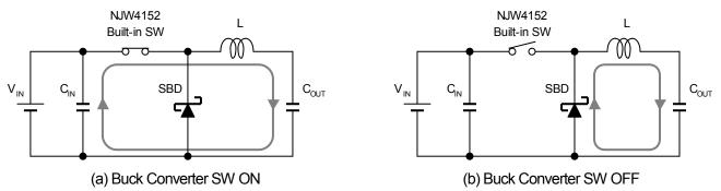
Fig. 5. Current Loop at Buck Converter
