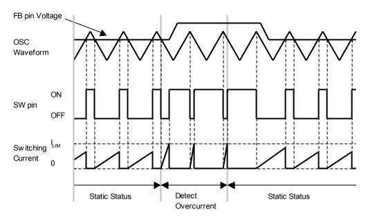
Fig. 3. Timing Chart at Over Current Detection
