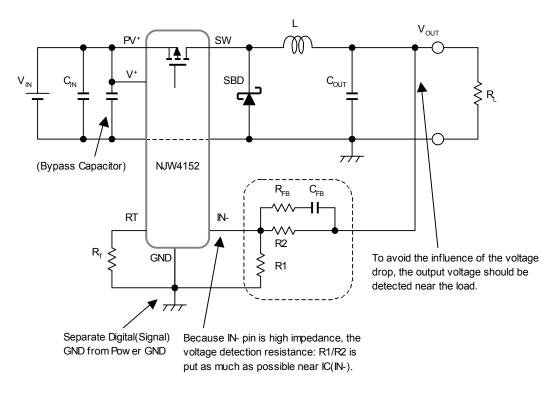
Fig. 6. Board Layout at Buck Converter
